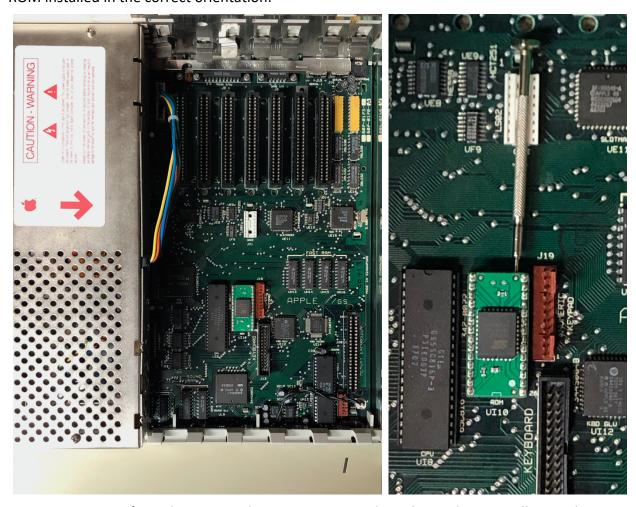
To remove a ROM from the ROM socket, we recommend gently wiggling a small screwdriver underneath the chip, alternating between the top and bottom, until the ROM can be gently removed, as shown above.
