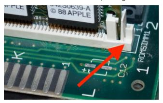
After identifying the type of ROM socket in your machine using the pictures above, select the correct set of reinforcing clips. If your ROM SIMM socket has metal tabs, you do not need to install the reinforcing clips. After installing the ROM SIMM itself into the socket, slide the correct type of clip over the edge of the ROM SIMM socket. First you may have to angle the reinforcing clip onto the side of the socket like so:
