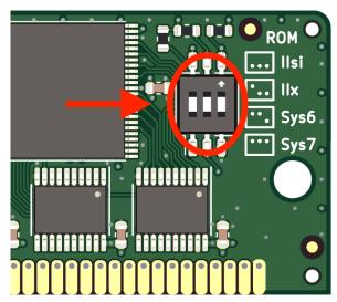
On Macintosh II-series machines, the ROM SIMM socket is accessible by just removing the computer's top cover. On Macintosh SE/30 machines, the computer must be disassembled and the motherboard removed in order to install the SIMM. Depending on your machine, a jumper may need to be installed or removed to enable the ROM disk.
