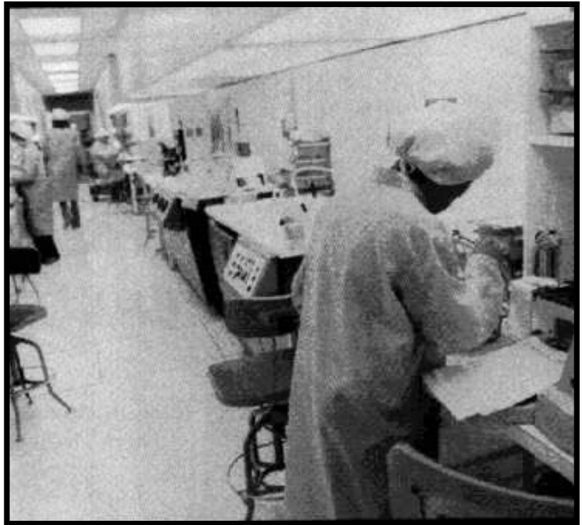
Photo 1: Processing. Photosensitized wafers are exposed with a particular mask pattern using ultraviolet light. The entire environment is otherwise ultraviolet-free.
