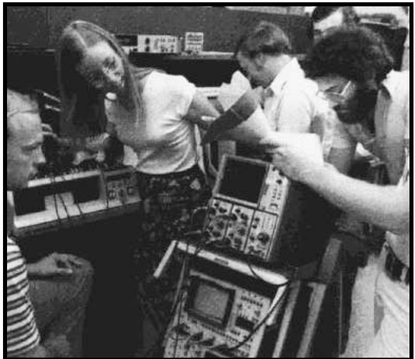
Photo 2: Breadboard debug. The gate level TTL model of the processor involves ten boards of 80 to 120 integrated circuits each. Many of the required 10,000 connections will be wrong. The system must be tested to find and correct construction and logic errors. Crowds are not unusual; here we have Don Tietjen, Katy Miller, James Tietjen, Steven Messinger (almost hidden), Mike Shapiro and Bill Keshlear.
