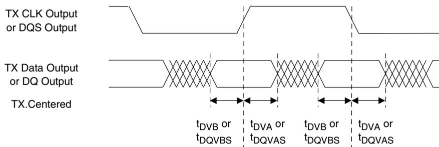
**Figure 3-9. GDDR71 Video Timing Waveforms**
