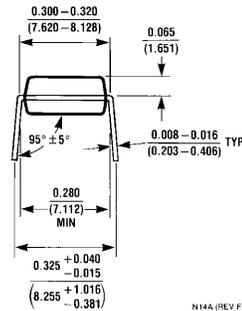
**14-Lead Molded Dual-In-Line Package (N)**
