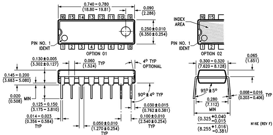
**16-Lead Molded Dual-In-Line Package (N)**
