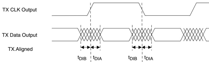
**Figure 3-8. Transmitter TX.CLK.Centered and MEM DDR Output Waveforms**
