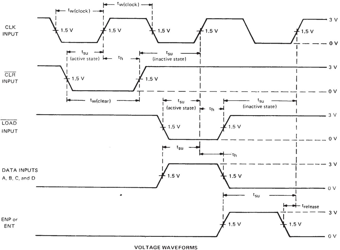
NOTE A: The input pulses are supplied by generators having the following characteristics:  $t_r \approx 2.5$  ns,  $t_f \approx 2.5$  ns, PRR = 1 MHz, duty cycle = 50%,  $Z_{out} \approx 50 \Omega$ .
