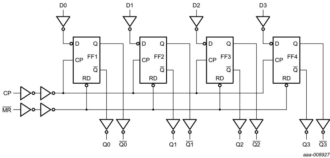
Fig 3. Logic diagram
