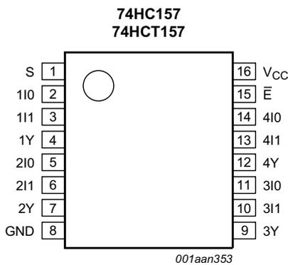
Fig 5. Pin configuration SO16, (T)SSOP16
