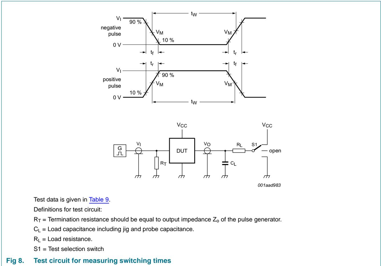
**Fig 8. Test circuit for measuring switching times**
