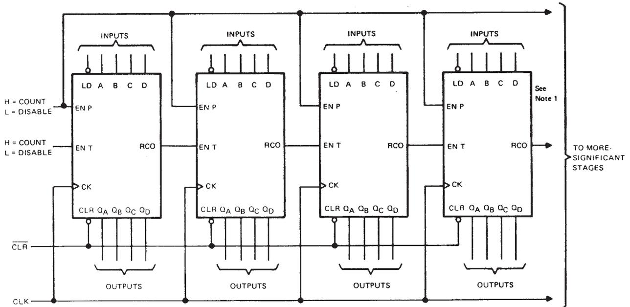
$$f_{MAX} = 1/(\text{CLK to RCO } t_{PLH}) + (\text{ENT to RCO } t_{PLH}) (N-2) + (\text{ENT } t_{SU})$$
