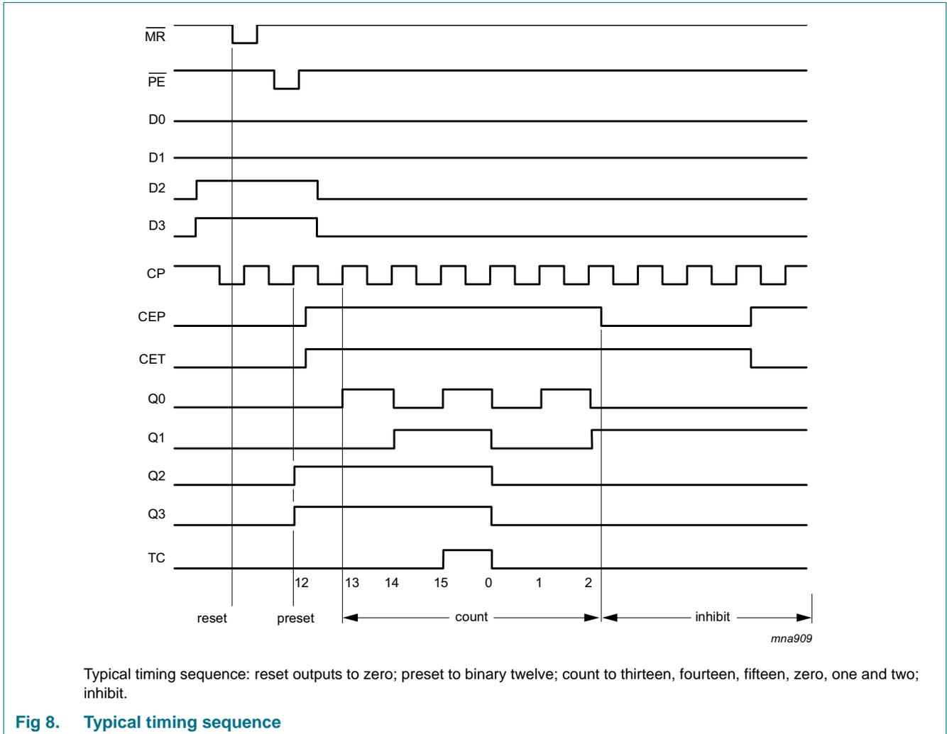
Fig 8. Typical timing sequence
