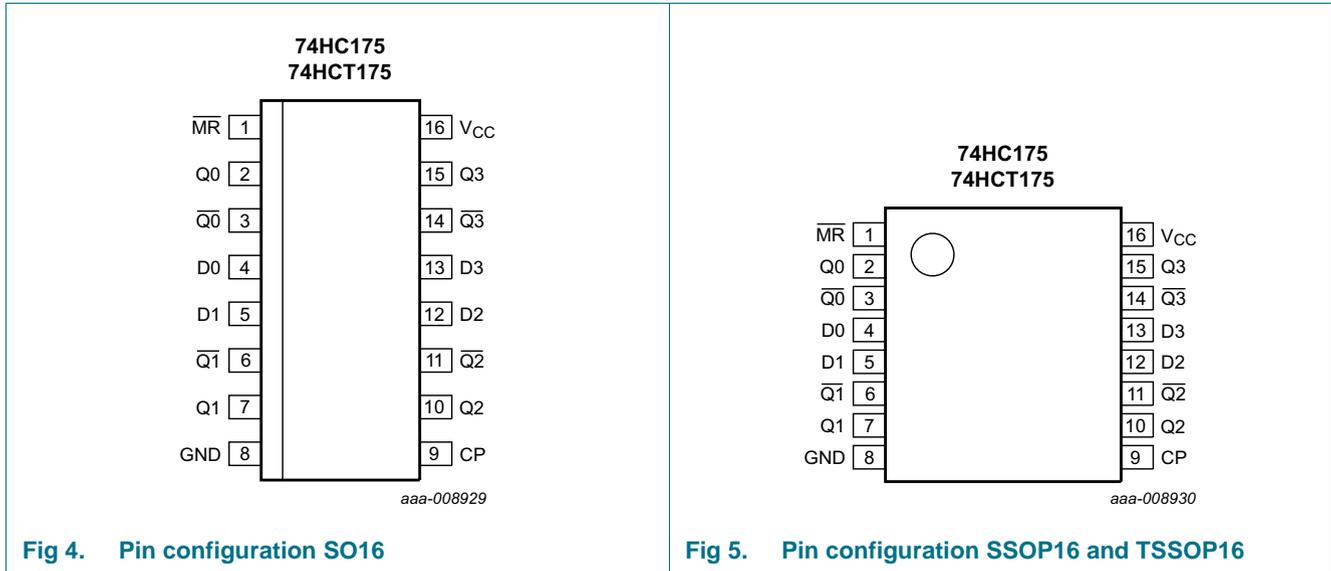
Fig 4. Pin configuration SO16
