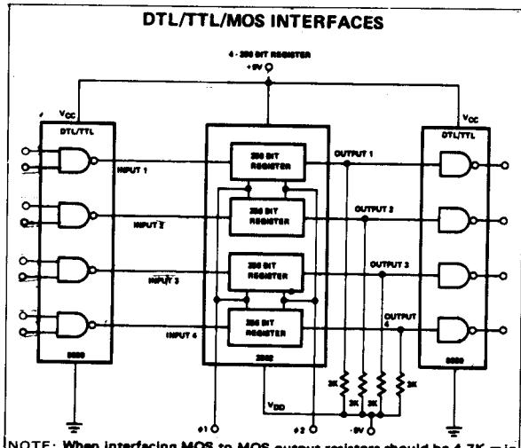
NOTE: When interfacing MOS to MOS output resistors should be 4.7K min
