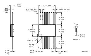
14-Lead Ceramic Flat Package (W) Order Number 54LS10FMQB or DM54LS10W Package Number W14B
