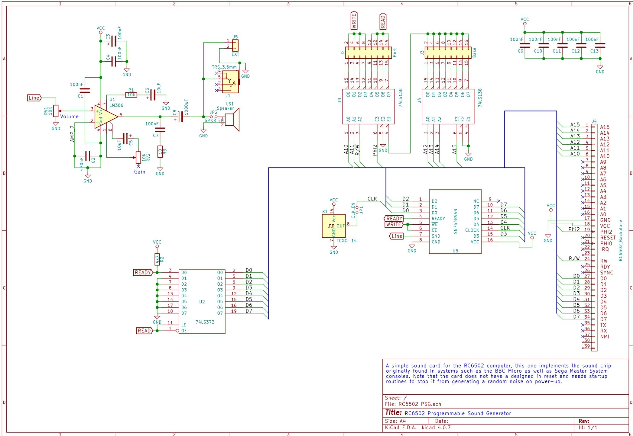
A simple sound card for the RC6502 computer, this one implements the sound chip originally found in systems such as the BBC Micro as well as Sega Master System consoles. Note that the card does not have a designed in reset and needs startup routines to stop it from generating a random noise on power-up.
