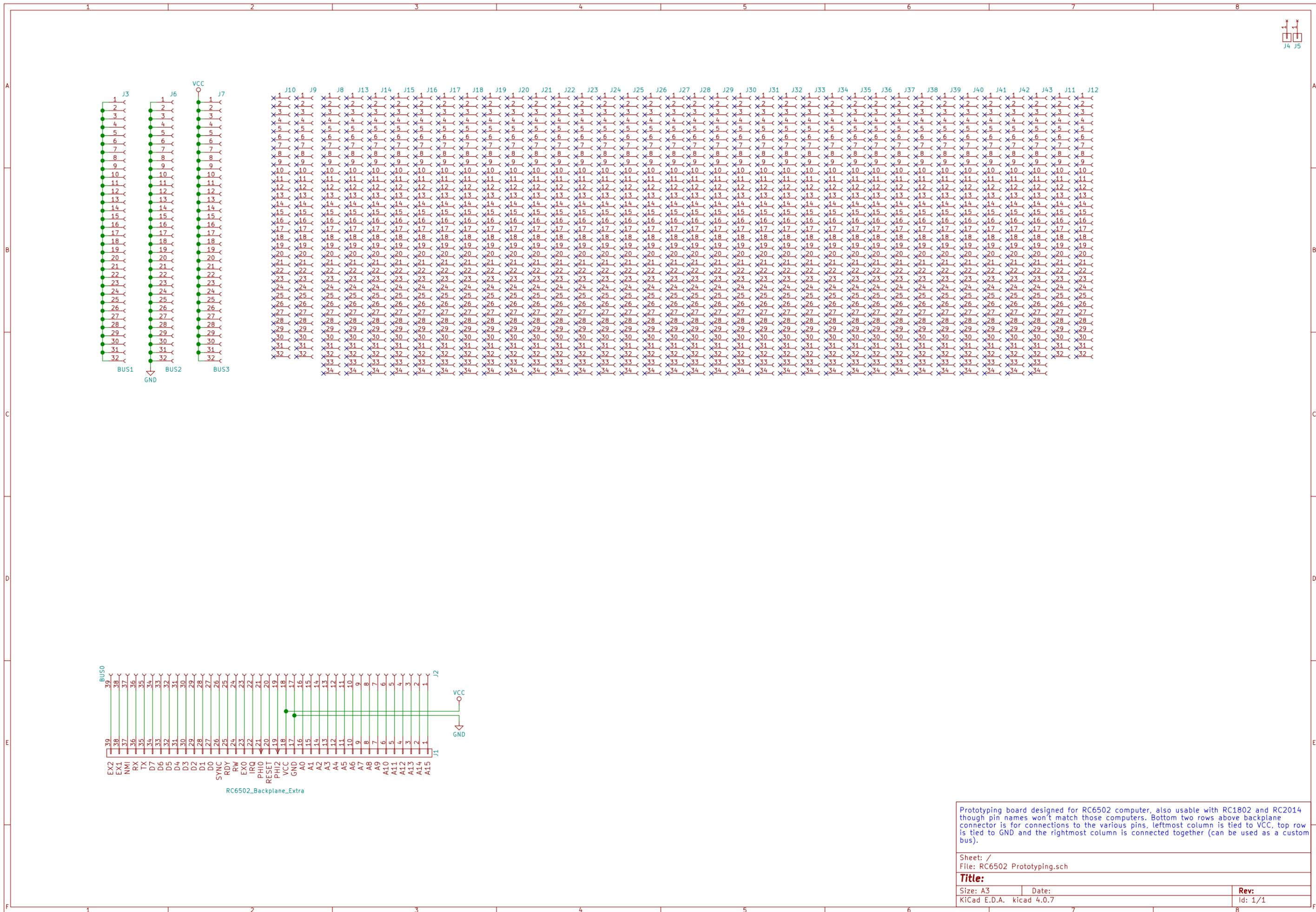
Prototyping board designed for RC6502 computer, also usable with RC1802 and RC2014 though pin names won't match those computers. Bottom two rows above backplane connector is for connections to the various pins, leftmost column is tied to VCC, top row is tied to GND and the rightmost column is connected together (can be used as a custom bus).
