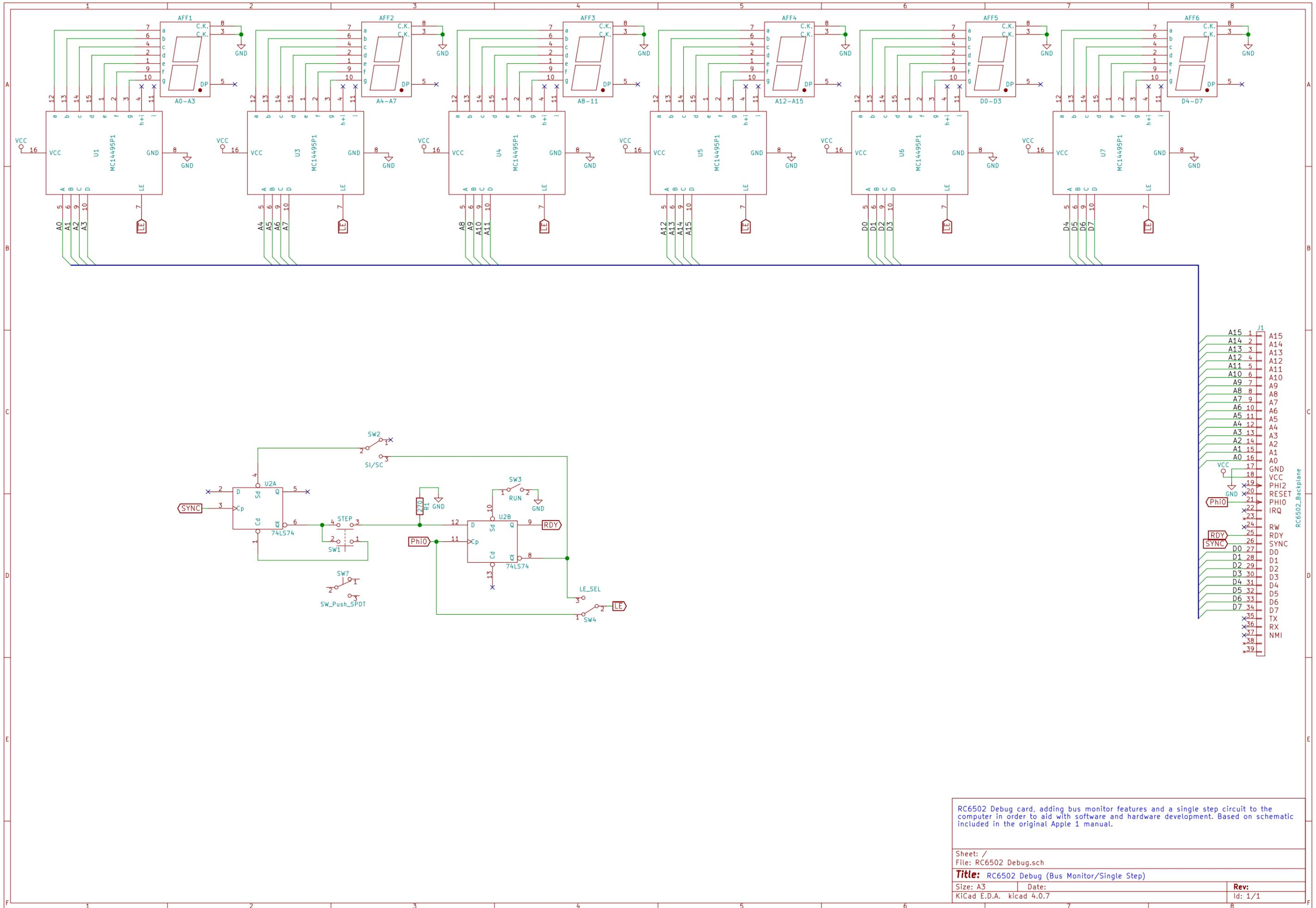
RC6502 Debug card, adding bus monitor features and a single step circuit to the computer in order to aid with software and hardware development. Based on schematic included in the original Apple 1 manual.
