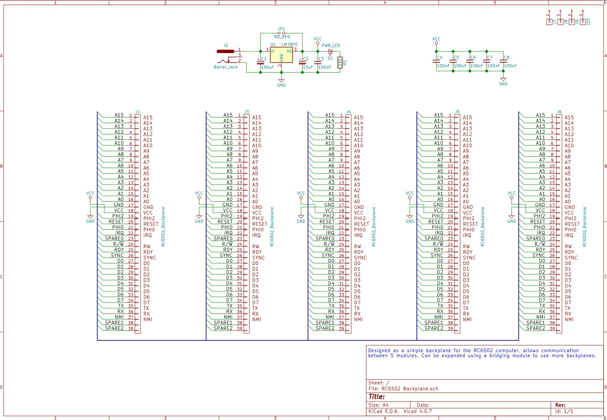
Designed as a simple backplane for the RC6502 computer, allows communication between 5 modules. Can be expanded using a bridging module to use more backplanes.
