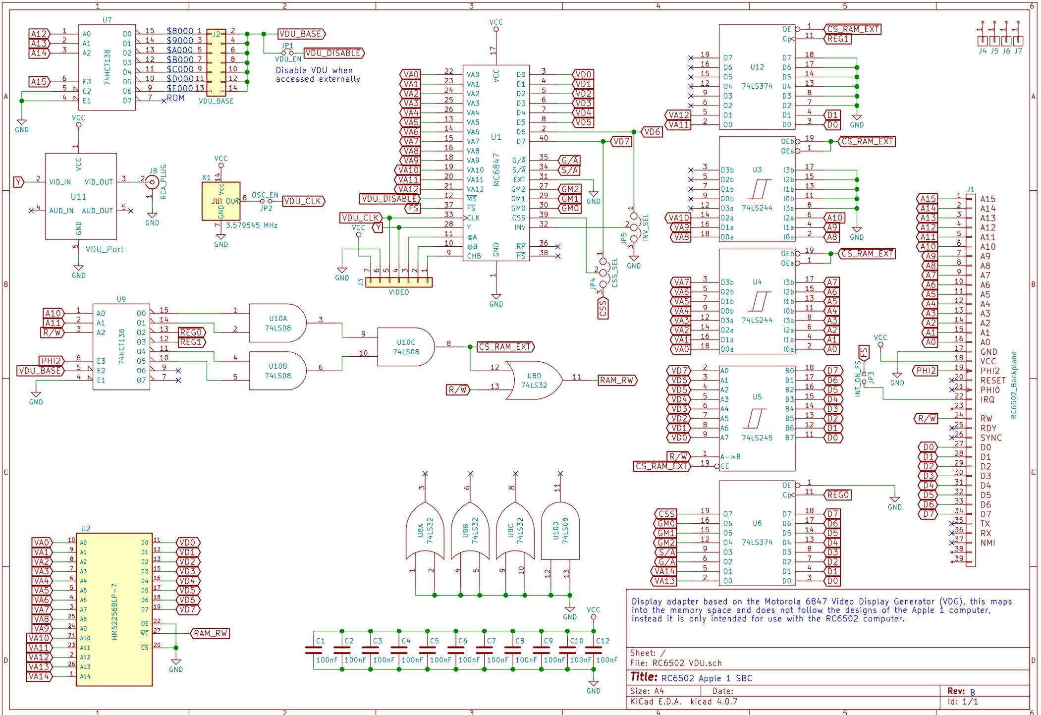
Display adapter based on the Motorola 6847 Video Display Generator (VDG), this maps into the memory space and does not follow the designs of the Apple 1 computer, instead it is only intended for use with the RC6502 computer.
