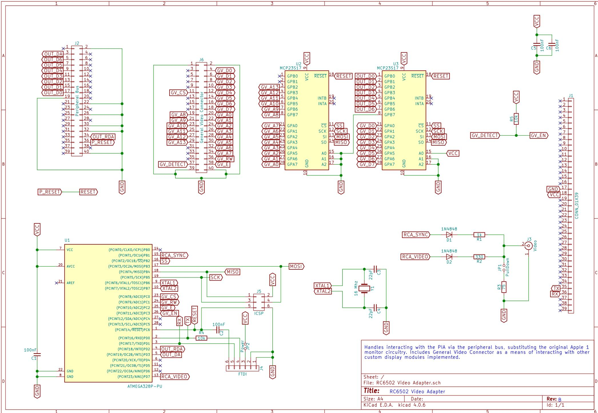
Handles interacting with the PIA via the peripheral bus, substituting the original Apple 1 monitor circuitry. Includes General Video Connector as a means of interacting with other custom display modules implemented.
