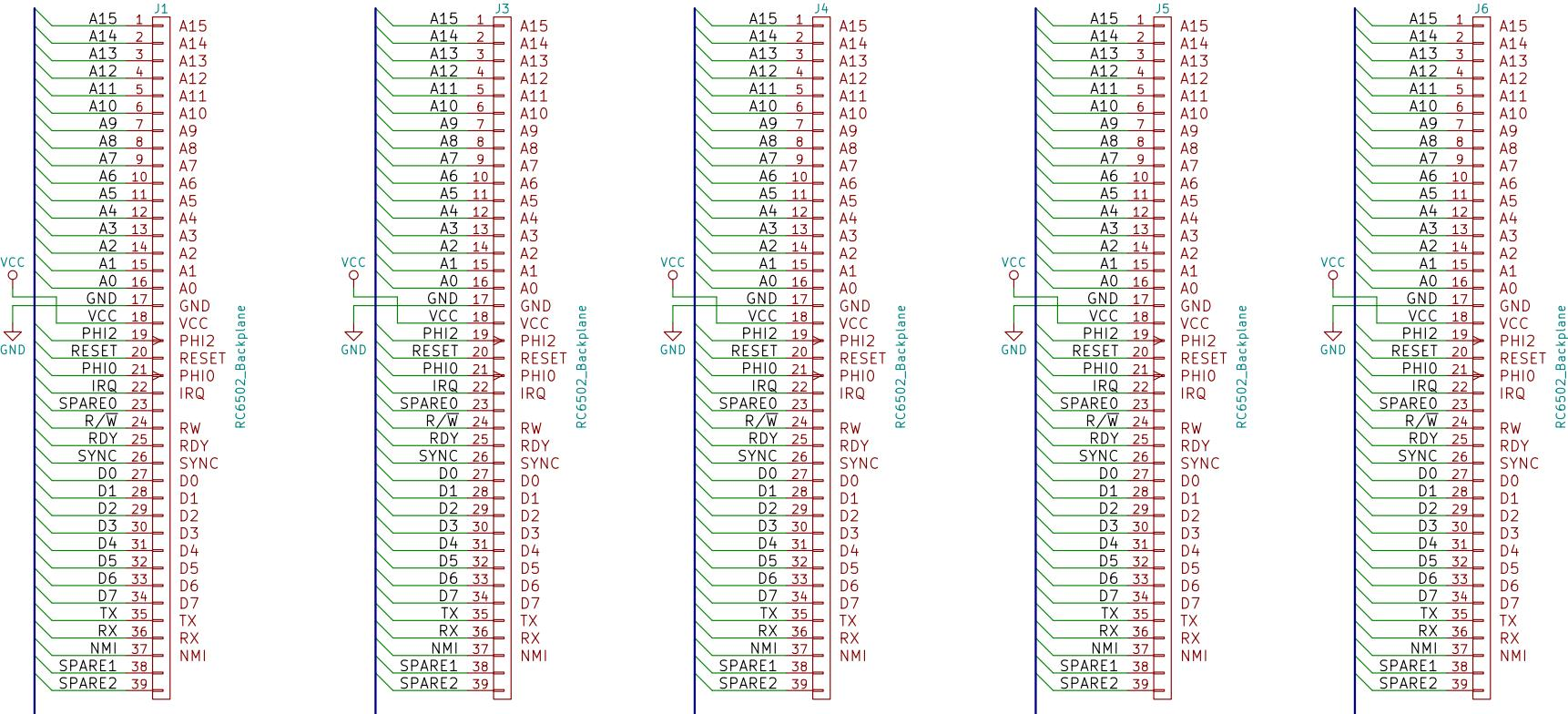
Designed as a simple backplane for the RC6502 computer, allows communication between 5 modules. Can be expanded using a bridging module to use more backplanes.
