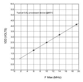
Figure 4-2a W65C22N F Max vs. VDD
