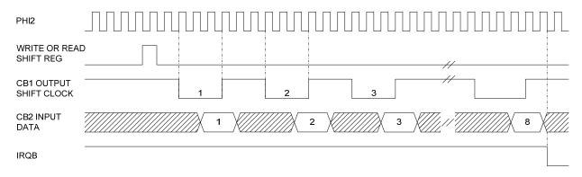
Figure 2-6 Shift In - Counter T2 Control
