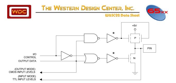
Figure 3-11 Rockwell - R65NC22 (CMOS), R6522 (NMOS) Port B Buffers (PB0-PB7)
