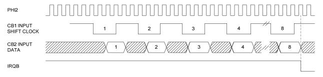
Figure 2-8 Shift In - External CB1 Clock Control Timing
