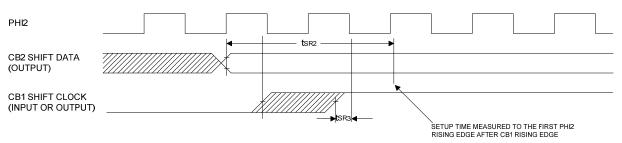
Figure 4-9 Data Shift In, Internal or External Shift Clock Timing
