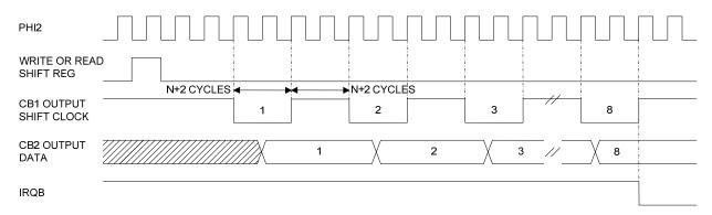
Figure 2-10 Shift Out - T2 Control Timing
