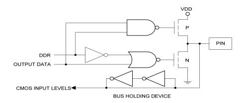
Figure 3-5 W65C22S Port A Buffer (PA0-PA7, CA2)
