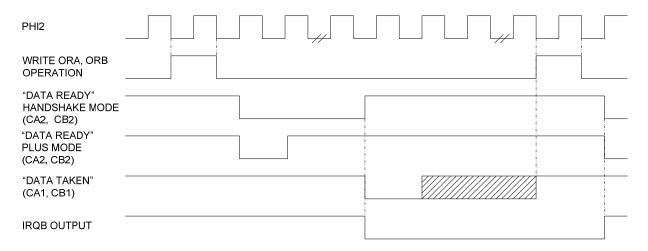
Figure 2-2 Write Handshake (PA and PB)
