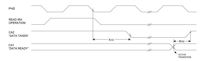
Figure 4-4 Read Handshake, Handshake Mode Timing (CA2)
