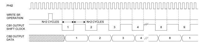
Figure 2-9 Shift Out - Free Running T2 Rate Timing
