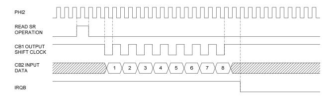
Figure 2-7 Shift In - PHI2 Clock Control
