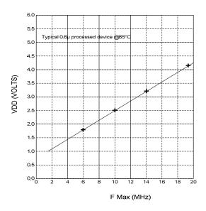
Figure 4-2b W65C22S F Max vs. VDD
