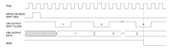
Figure 2-12 Shift Out - External CB1 Clock Control Timing
