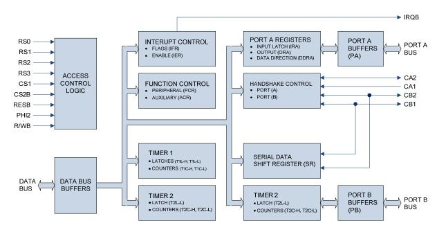
Figure 1-1 W65C22 Internal Architecture Block Diagram
