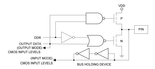
Figure 3-9 W65C22S Port B Buffer (PB0-PB7, CB1, and CB2)
