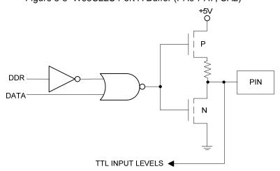
Figure 3-4 W65C22N and GTE - G65SC22 CMOS Port A Buffer (PA0-PA7, CA2)
