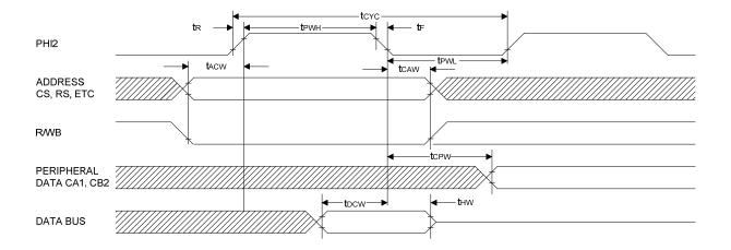
Figure 4-2 Write Timing
