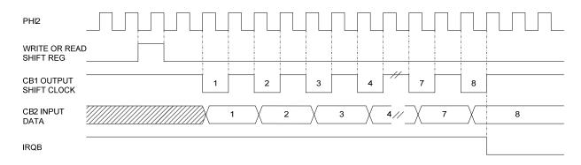
Figure 2-11 Shift Out - PHI2 Control Timing
