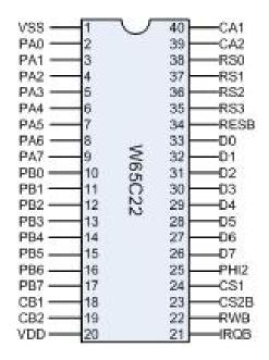
Figure 3-1 W65C22 40 Pin PDIP Pinout
