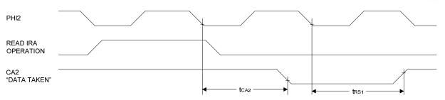
Figure 4-3 Read Handshake, Pulse Mode (CA2)
