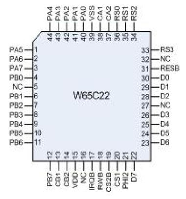
Figure 3-3 W65C22 44 Pin QFP Pinout
