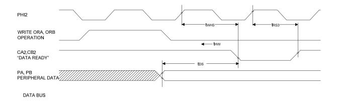
Figure 4-5 Write Handshake, Pulse Mode Timing (CA2, CB2)
