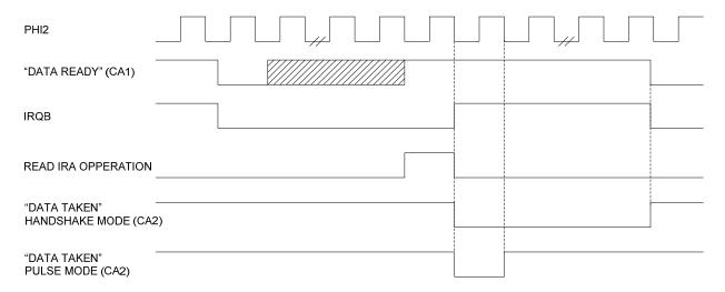
Figure 2-1 Read Handshake Operation (PA Only)
