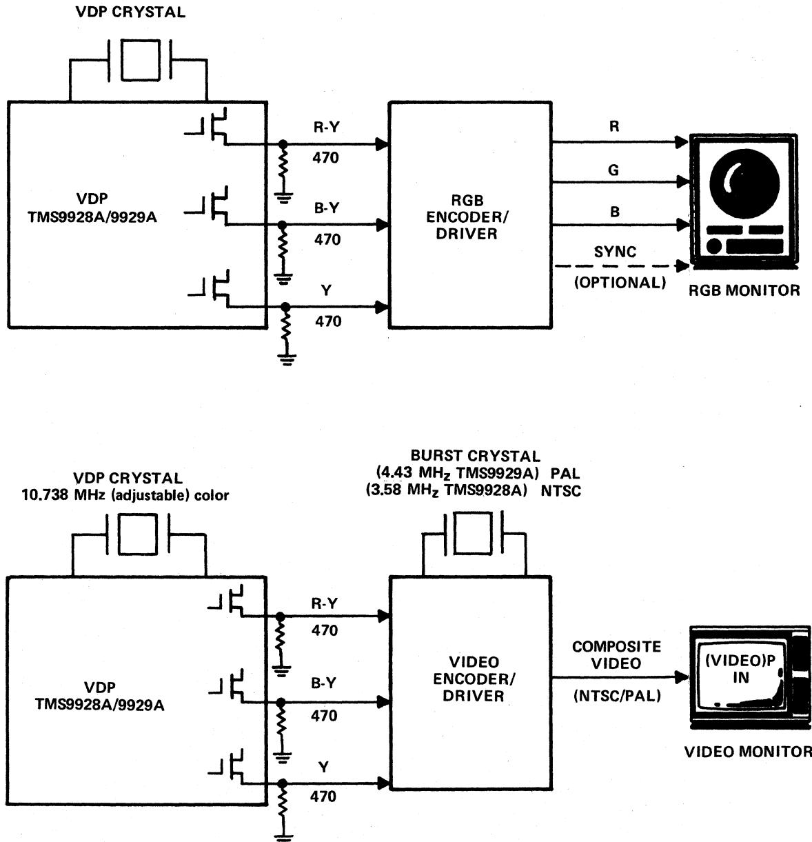
NOTE: The LM1889 is typically used in the video encoder circuitry.
