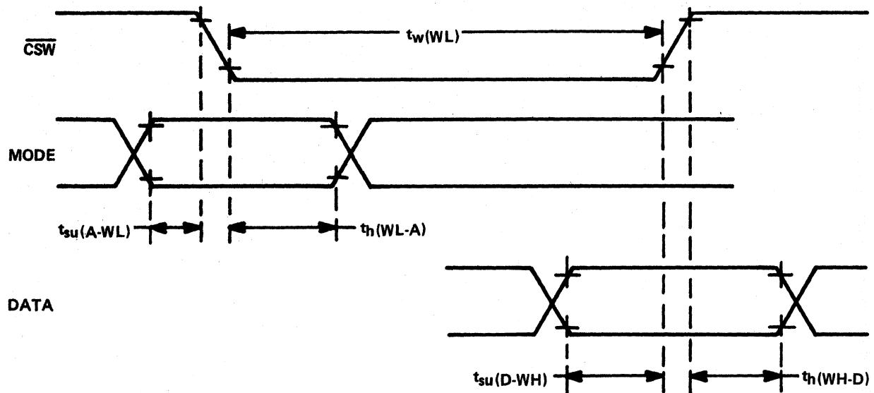
FIGURE 5-3 – CPU-VDP WRITE CYCLE FOR TMS9918A/9928A/9929A
