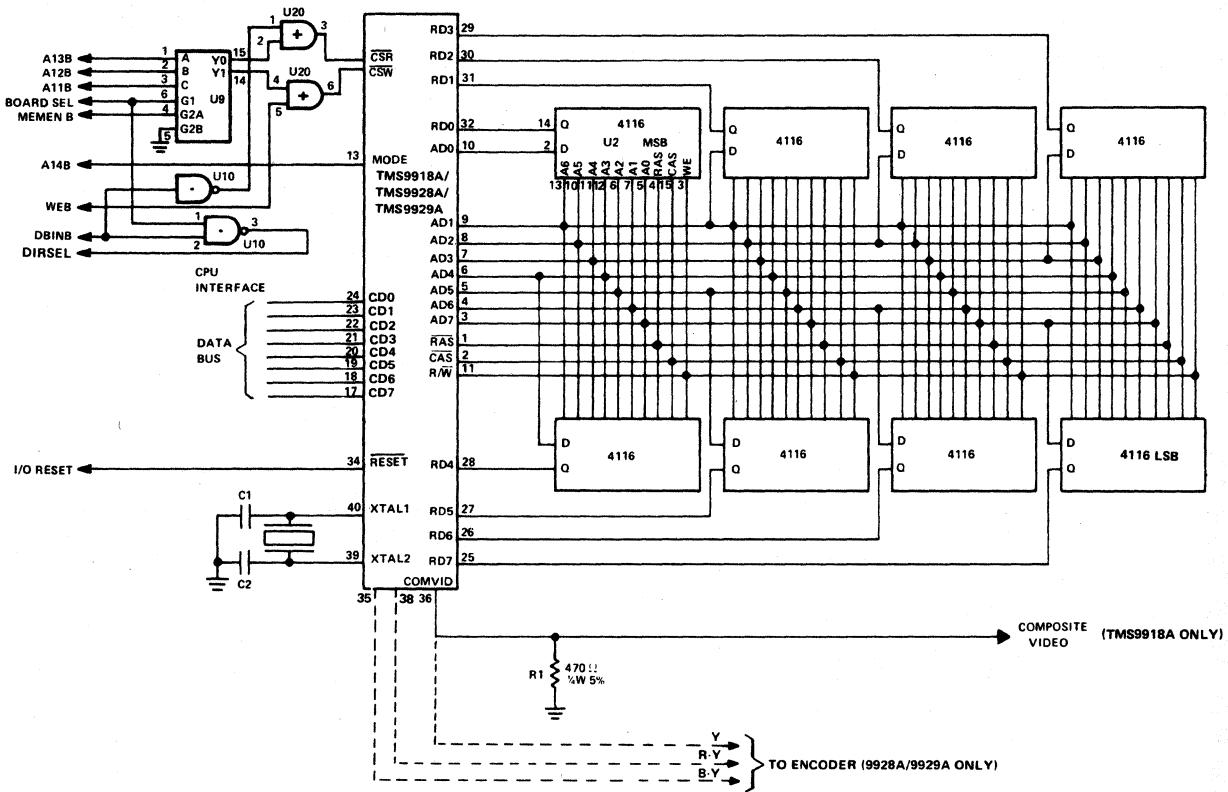
FIGURE 4-2 — TMS9918A/9928A/9929A INTERFACE
