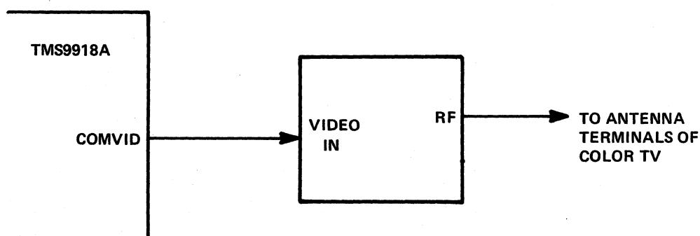
FIGURE 4-4 — RF MODULATOR CONNECTION
