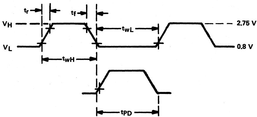
NOTE: All measurements are made at 10% and 90% points.
