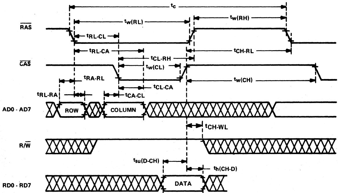
NOTE: All measurements are made at 10% and 90% points.
