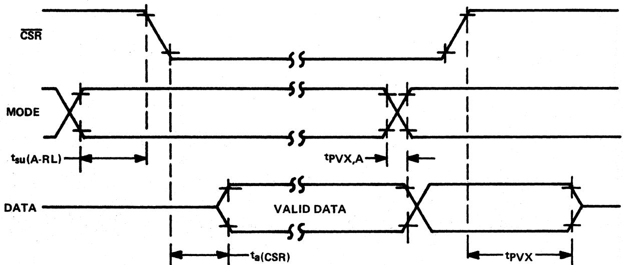
NOTE: All measurements are made at 10% and 90% points.
