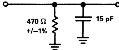
**FIGURE 5-1 – LOAD CIRCUIT FOR COMVID (ALL DEVICES) AND R-Y, Y,
