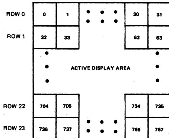
FIGURE 2-9 — PATTERN GRAPHICS NAME TABLE MAPPING
