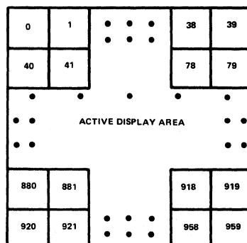
FIGURE 2-17 — TEXT MODE NAME TABLE PATTERN POSITIONS
