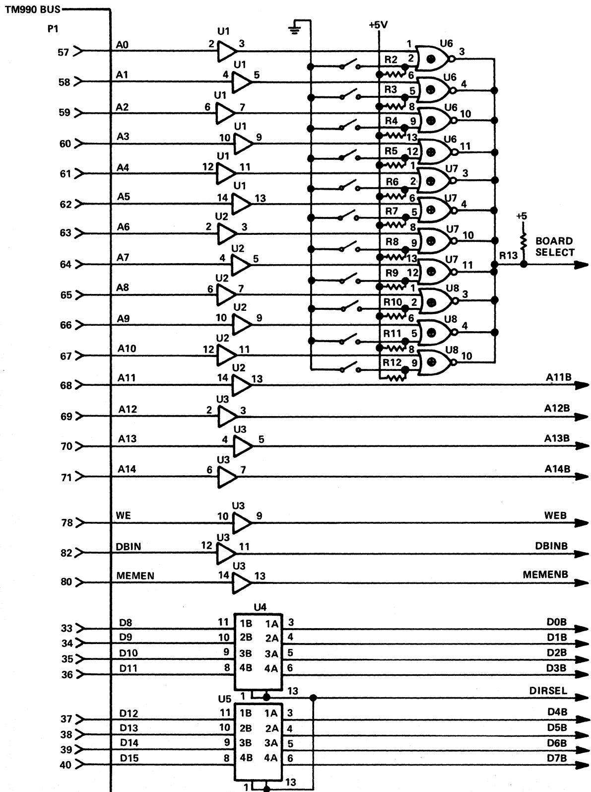
FIGURE 4-3 — TM990 (TMS9918A/9928A/9929A) DEMO BOARD
