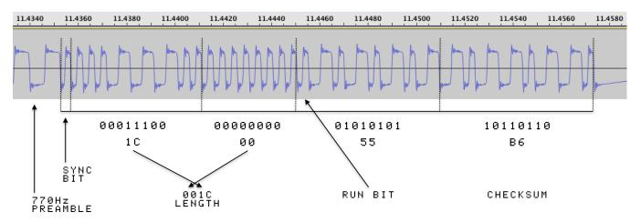
Figure 1 illustrates the header for a small FP BASIC program that I captured using the BASIC SAVE command. What you do not see left of the SYNC Bit is 10 seconds of 770 Hz tone and about 1.4 seconds of nothing (first had to press record on my recorder and then type "SAVE" and press RETURN-- that took about 1.4 seconds). Each bit is represented by a full cycle square wave. Narrow bits (the zeroes) have higher frequencies (2000 Hz) and wider bits (the ones) have lower frequencies (1000 Hz).
