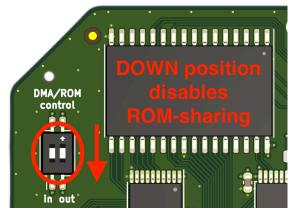
switches on the card should be set to the lower position (further away from the "ON" text). With both switches in the upper position, the ROM-sharing functionality is enabled.
