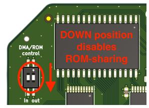
switches on the card should be set to the lower position (further away from the "ON" text). With both switches in the upper position, the ROM-sharing functionality is enabled.
