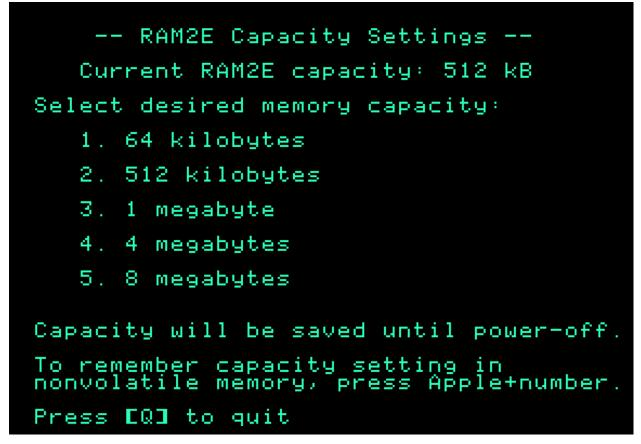
For example, by pressing the "1" key, the capacity can be set to 64 kilobytes until the computer is powered off. By pressing Apple+1 (open-Apple or closed-Apple), the 64 kilobyte capacity setting can be saved in nonvolatile memory as well, so that it is restored on power-up.
