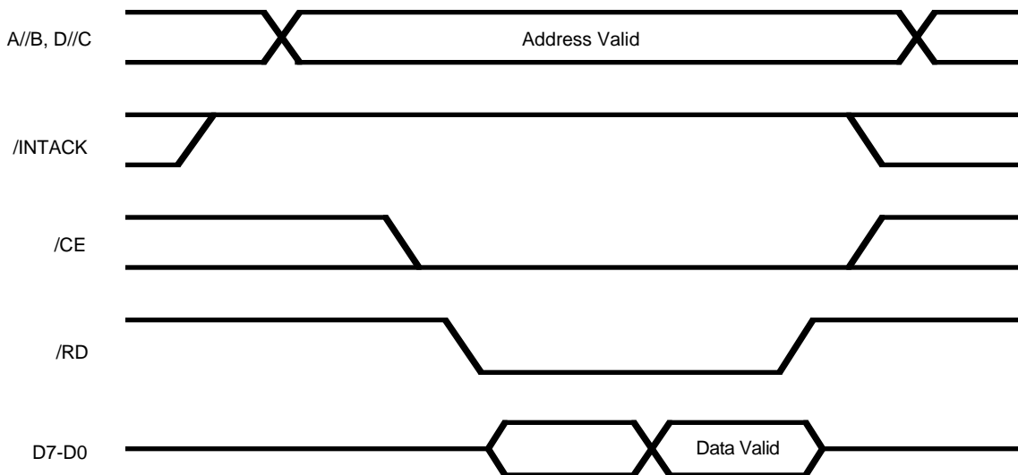
Figure 2-5. Z85X30 Read Cycle Timing
