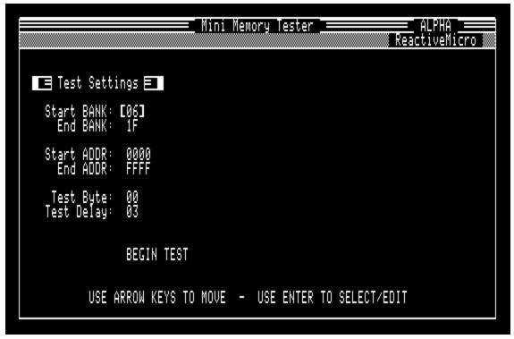
Using the up and down arrows, you can select which menu item you want (indicated with square brackets), and hit enter to edit it, or if "BEGIN TEST" is selected, it will of course begin testing memory using your specified parameters.
