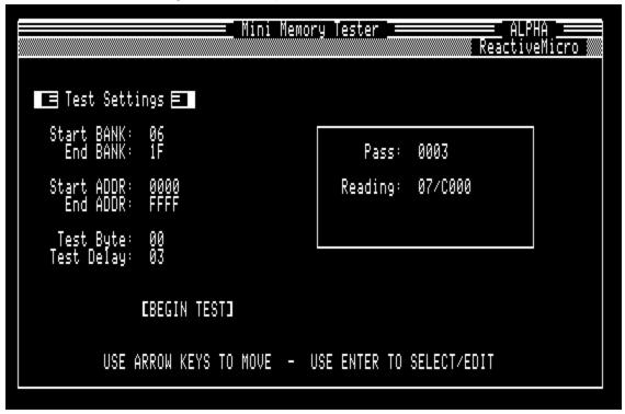
After each pass of writing and reading, the pass number is incremented, and the next pass starts.
