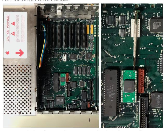
To remove a ROM from the ROM socket, we recommend gently wiggling a screwdriver underneath the chip, alternating between the top and bottom, until the ROM can be gently removed, as shown above.
