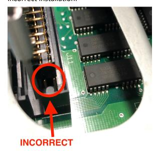
After ensuring that the card is correctly aligned with the connector pins on the Macintosh motherboard, press firmly downward to secure the RAM card in place.
