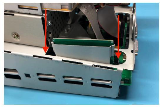
Ensure that the card is aligned correctly with the connector on the motherboard. Make sure the card is aligned correctly with the pins on the motherboard's slot such that all the pins are inserted into the card's connector.
