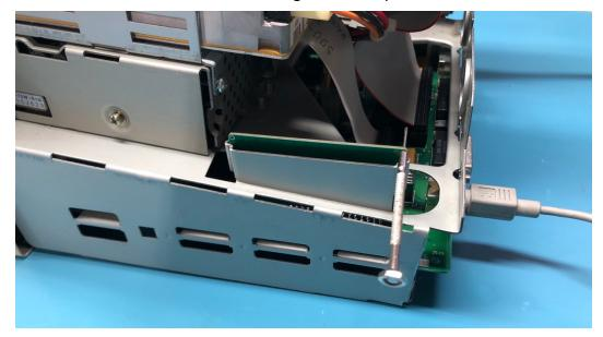
Pull the board upward using the screwdriver, alternating between the two mounting holes, until the board is loose in the socket and can removed by hand.
