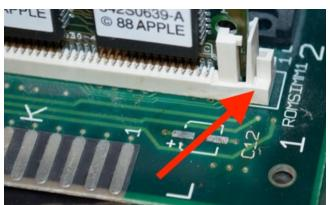
After identifying the type of ROM socket in your machine using the pictures above, select the correct set of reinforcing clips. If your ROM SIMM socket has metal tabs, you do not need to install the reinforcing clips. After installing the ROM SIMM itself into the socket, slide the correct type of clip over the edge of the ROM SIMM socket. First you may have to angle the reinforcing clip onto the side of the socket like so:
