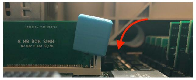
Then push down to slide the clip downward until the clip is fully seated on the SIMM socket:
