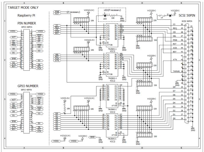
This is a circuit diagram example of a conversion board that supports target mode (HDD, MO, CD, etc.) and initiator mode (host function). I use three more GPIOs. The direction control of all 74LS641-1 is controlled from the RaSCSI side.
