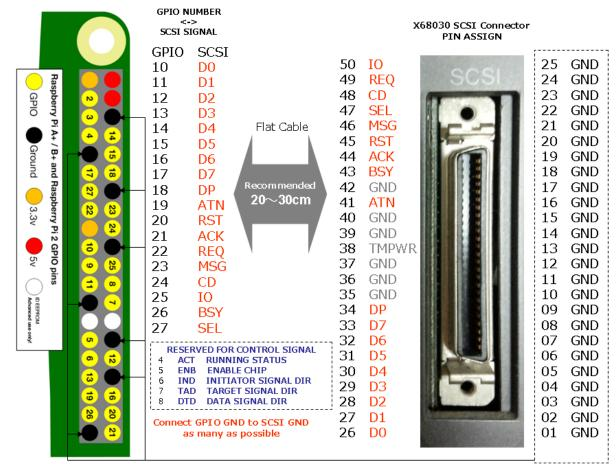
is stable if you pull out as many GND as possible on the SCSI connector side (8 if possible) and connect it to the GND on the RPI side. It seems to do.
