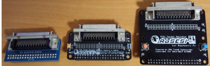
There is also a direct connection board. Basically it is the same as the direct connection cable, but it seems that there is no problem if you use a SCSI cable because it is easy to electrically stabilize.
