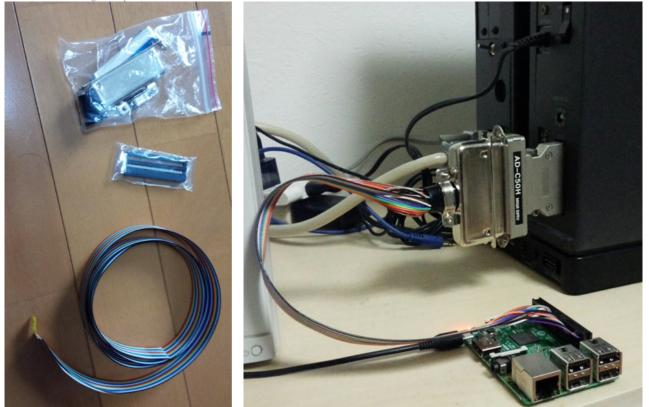
material used was a 40-pin MIL connector, Centronics 50-pin male, and flat cable. It is recommended to keep the flat cable within 30 cm (the length is longer than this and there is no actual result). The SCSI connector will be half size male (ribbon type) for X68030 and XVI Compact, and full size male for other SCSI machines. You can also use a conversion adapter as shown in the photo. GPIP pins aren't lined up neatly, and I'm using different pins to
