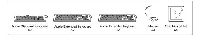
In the example shown in Figure 5-6, all three keyboards are the same device type; thus, they share the same default ADB device address (\$2). When the ADB Manager begins to build the device table by sending a Talk Register 3 command to address \$2, all three
