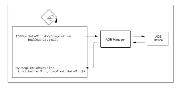
Listing 5-2 shows a way to send ADB commands synchronously.
