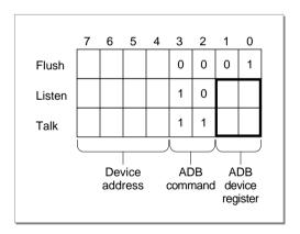
Bits 0 through 1 specify the ADB device register, bits 2 through 3 specify the command code, and bits 4 through 7 specify the device address.
