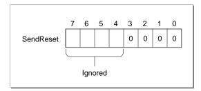
The first four bits of the SendReset command identify this command. Because the SendReset command applies to all ADB devices, bits 4 through 7 do not specify the address of a particular device. As previously described, an ADB device never receives a SendReset command; instead, the device resets itself in response to the 3 millisecond pulse.
