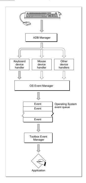
The ADB Manager retrieves data from an ADB device as a result of its normal polling process. The ADB Manager polls a device by sending it a command requesting it to return the contents of one of its registers. (Note that an ADB device should respond to the specific ADB command, Talk Register 0, only if the device has new data to send. See the next section, "ADB Commands," for more information.)
